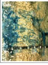
Fig. 4. Profile (in centimeters) displaying the infiltration test result of the natural undisturbed horizons of a soil in Hydrologic Soil Group C.
