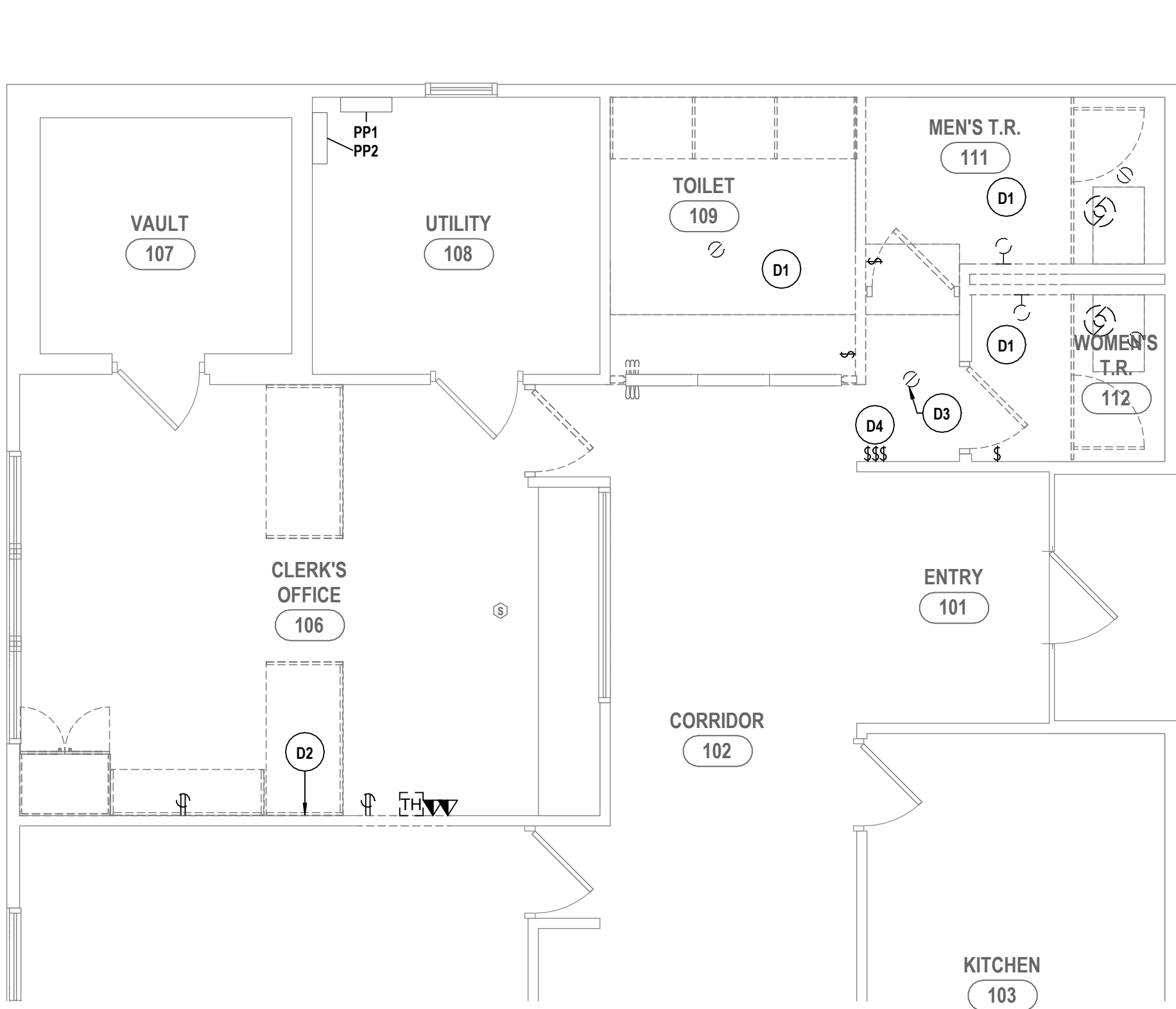
1 PARTIAL FIRST FLOOR ELECTRICAL DEMOLITION PLAN 1/4" = 1'-0"
