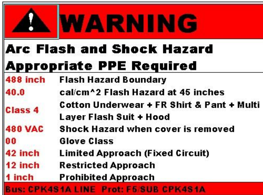
Example of Arc Flash Warning Label
