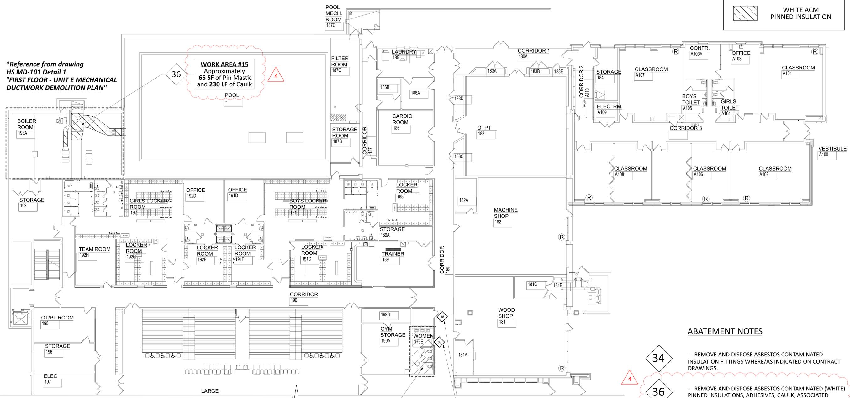
*\*Reference from drawing HS MD-101 Detail 1 "FIRST FLOOR - UNIT E MECHANICAL DUCTWORK DEMOLITION PLAN"*
