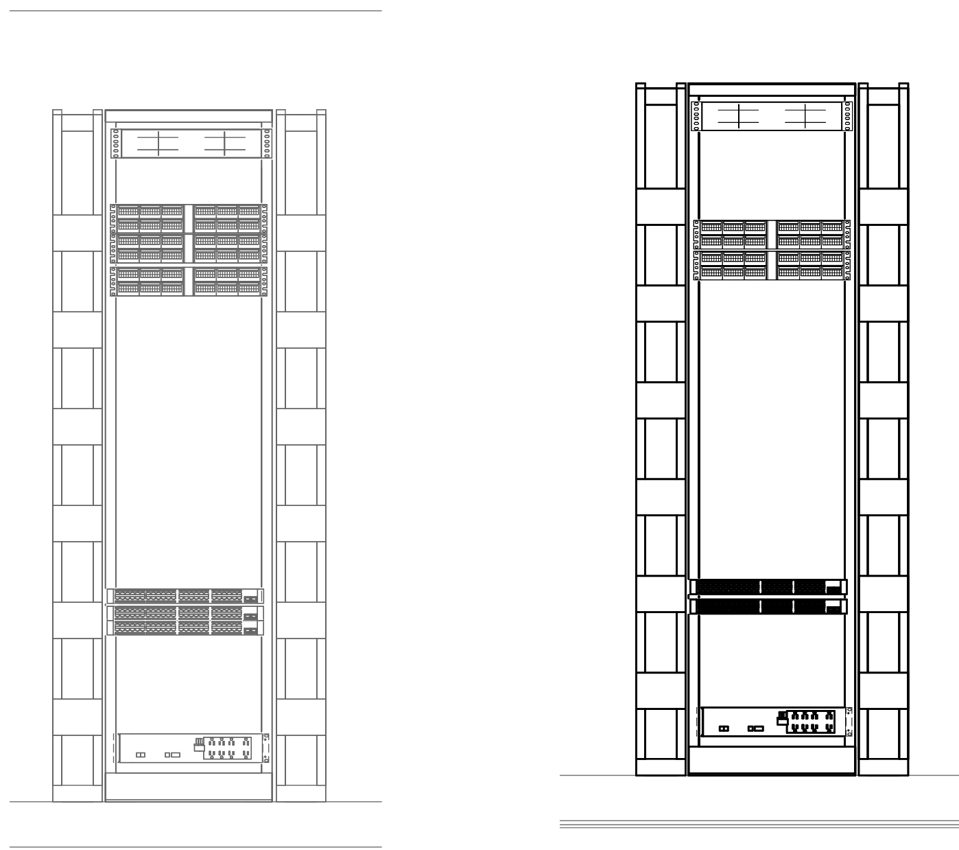
4 MDF 237 RACK 2 ELEVATION VIEW 3/4" = 1'-0"
