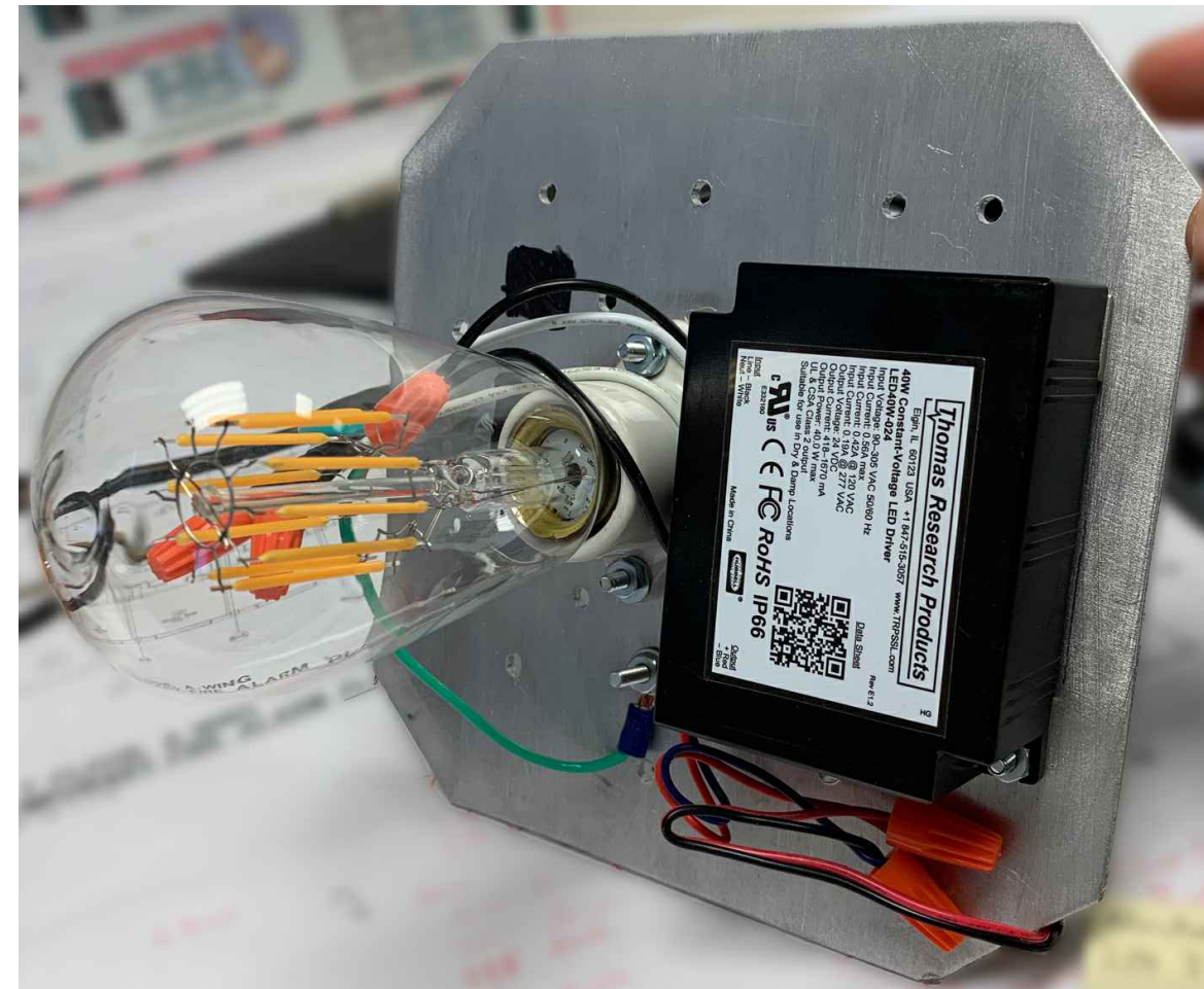
9 E220 LAMP ASSEMBLY MOCKUP: BOTTOM VIEW NOT TO SCALE
