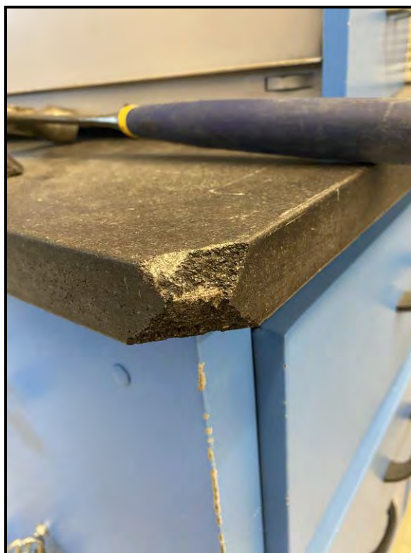
HA 02 – Counter-top, Room 309, “No Asbestos Detected”
