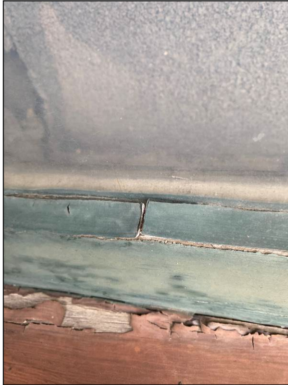
HA 05 – Window Glazing Compound, “No Asbestos Detected”
