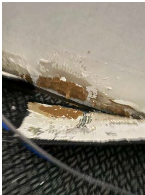
White Mastic from various colors of Non-Suspect Vinyl Cove Base, No Asbestos Detected Typical for HA's 02, 04 & 07
